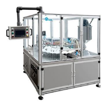
This machine is designed for cream products in jar, it includes auto feeding, auto inner seal, auto outer cap feeding, and auto capping system.
