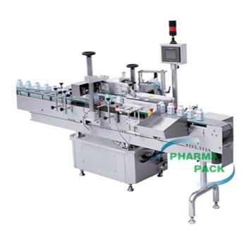
The label strip from the label roll holder is spread around several guiding rollers, through the dispenser and fixed on the base paper recycle roller lastly. Bottles are fed via the spacing wheel. When the sensor detects the coming bottle, it will signal the label dispenser to stick out a piece of label, which is stripped off by the passing bottle. Then the label will be pressed closely against the bottle surface by the label wrapping device.
