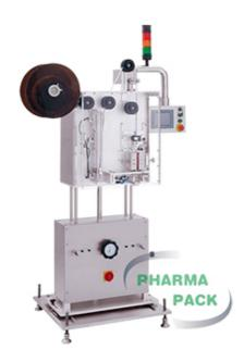
The desiccants strip on the roll holder is routed through several guiding wheels, through the length verification device and into the dispenser. Once the machine starts, the dispenser feeds a preset length of the desiccant strip with the help of the servo motor. If the actual length is confirmed as the setting by the length verification device the desiccant sachet will be cut by the cutter and drop into the bottle via the nozzle.
