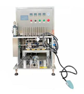
KIS-1 Desktop Aluminum Cup Pre-cut Aluminium Foil Sealing Machine is a tabletop model with heat sealing features. Very compact, it is a drawer style cup sealer that seals pre-cut aluminum foil with a pneumatic piston. As you push in the drawer holding your food-filled cups, the machine seals over the cups.
