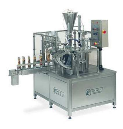
Pouches are the most reliable packing method for juices, dairy products, salad dressing, soups, spices, detergents and more. PDP-4 is a rotary pouch packaging machine designed on a mechanical rotary platform base with pneumatic assemblies. Extreme flexibility is the machines' greatest asset. The lines operate with fillers for liquid, dry or powdered paste and hot products. The machine adjustments for different pouch sizes are fast and easy.
