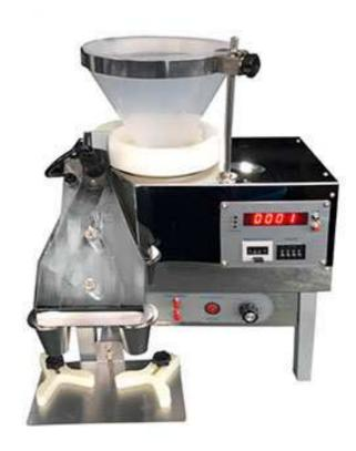
The counting machine is a kind of machine which is suitable for counting drugs or food such as capsules, tablets and particles in pharmaceutical, hospital and food industries. Advantages The machine is small in size, light in weight, accurate in counting and easy to operate. The machine is made of stainless steel and CE certified.
