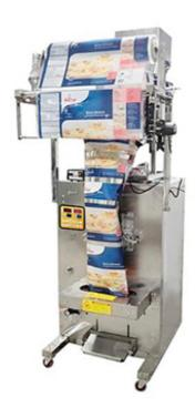
3kg, 5kg large food grain rice beans sugar spices dried pepper powder packing machine, accurate measurement, multi-functional packaging machine, automatic packaging and tight sealing.
