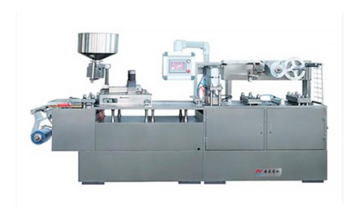
It is the latest generation product in our company which adopting PLC Human interface operation, with frequency Converter, high automation, easy operation, novel figure, all-round-functions, advanced technology, stable running, durable life, qualified with GMP. It is an ideal blister packing machine for AL-plastic, paper-plastic and it has got high popularity.
