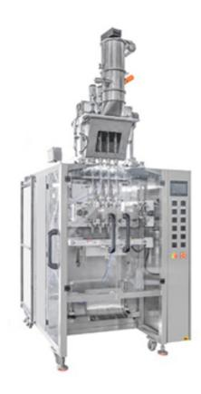
4 lane Powder stick pack Machine that is suitable for packing fine dry powder materials, such as milk powder, spices powder, coffee powder, corn flour, laundry powder, coconut powder, fruit powder, collagen protein powder, cocoa powder, chili powder, etc.
