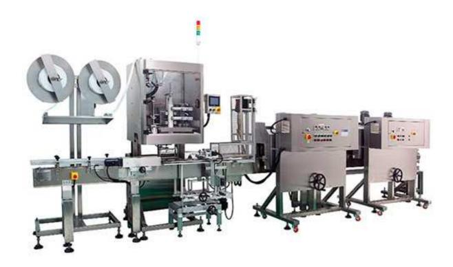
Auto Body Label Sleeve Applicator, LG-150 is designed matching CE certificate, higher safe standard. Machine is designed with SUS frame to match production requirement of Foods & Pharmaceutical industries.
