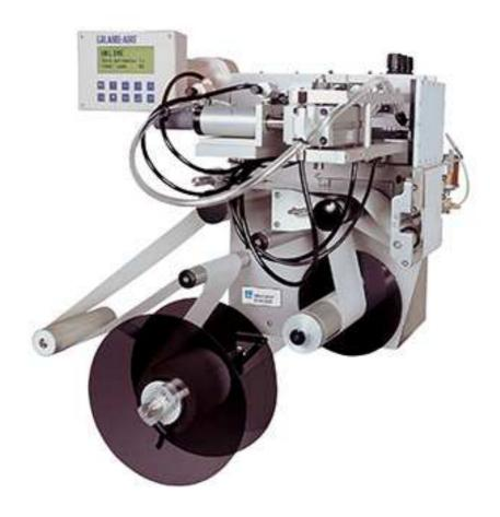
The Label-Aire Model 3114 Label Applicator represents the ultimate in dual action tamp pressuresensitive labeling technology.
