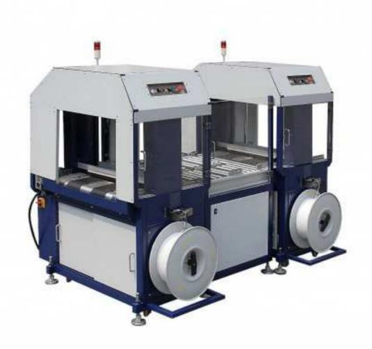
The strapping machine takes polythene plastic strap as binding material, which is mainly used in packing and binding of paper carton, wooden box and paper and paper parcels in sectors of business, postal service, railway, bank, food, pharmaceutical and publishing.
