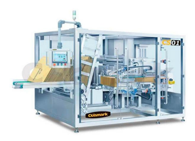
Colamark Case packer integrated Case feeder, Case erector, product insertion, Case closing in one machine. Optional card board and leaflet insertion, Camera Track and trace feature and outer case printing/labeling are available to maximize your investment. As space is always a concern on production floor, our All-In-One design case packer can offer multi-functions on single machine with synchronization of other Colamark upstream machines.
