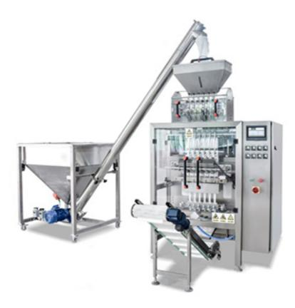
Multi Lane Grain sick packaging Machine is suitable for many kinds of loose granule products, such as sugar, salt, small grains, seeds, spice, etc.
