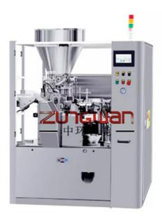
Tube filling and sealing machine is used for filling of polyethylene and laminated tubes with gels, creams or other fluids, sealing them with hot air.
