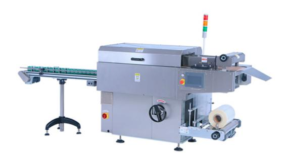
The Overwrapper is an End-of-Line Packaging Machine. It groups cartons (or similarly shaped objects) together or stacks them in bundles, and tightly wraps them in the film leaving excess material at either end. The excess film at the ends of the bundle is then folded and sealed. All-around sealing further enhances the moisture-proofing of the product. It also can be connected to a packaging line with Blister Machines, Cartoners, and Case Packers.
