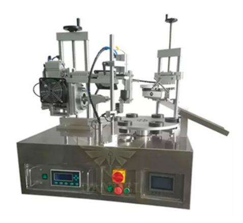
The process of tube sealing machine eliminates the use of glue and allows the thermoplastic parts to bond to itself. Ultrasonic sealing with the proper time setting and pressure is the fastest most reliable method for a variety of tube material sealing.
