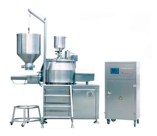
This Vertical Granulators have a long history in the pharmaceutical industry, they are always first choice when the process needs high granulate density and rapid granulation. In addition, they have low space requirements, are simple to operate and easy to clean.
