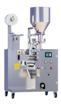
It is suitable for packing instant noodles soup bag, desiccant, tea power, small granular materials. The machine can finish bag making, measuring, filling, sealing, cutting and counting functions automatically.
