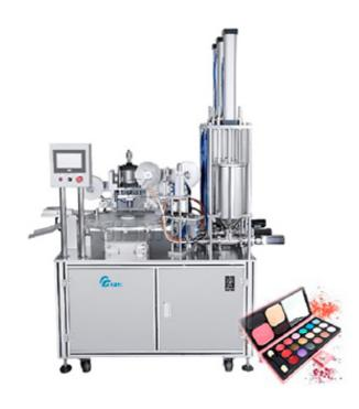
This machines is designed for extruding and forming 3D baked powder and blusher
