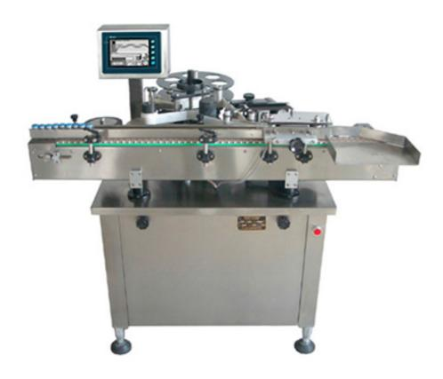
DLTB-C is economical, self contained, easy to operate, equipped with auto teach programming touch screen. Built in microchip storing different job setting makes fast and easy changeover.
