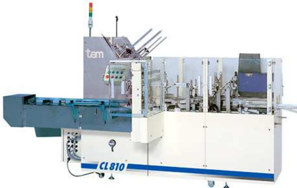
CL810 Cartoner is our intermittent cartoner that comes in a compact size. The blank carton sheet is picked from carton magazine and formed automatically, then products are inserted holistically and flaps are closed. The customer can choose to have cartons either glued or tucked. Automatic insertion device can be equipped for line-production.
