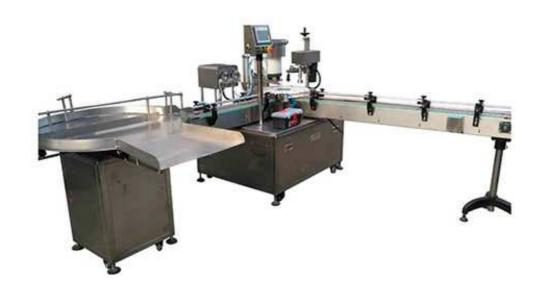
The automatic spray bottle filling capping machine is mainly designed for plastic or glass round and flat spray bottles and suitable for filling liquid like cleaner liquid spray, surfactant, medicinal spray, nasal, hair wax, serum, air freshener, cream, lotion and so on. The spray bottle filling machine adopts the peristaltic pump or piston pump metering with the filling range 20-200ml, high precision.
