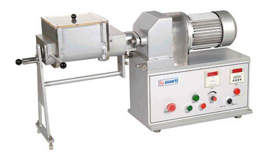
The Lab Mass Mixer having horizontal half round bowl open on the upper side with acrylic cover and specially designed mixing blade. The Main Mixing Blade is rotated to circulate the material to be mixed. The half-round bowl and mixing blade made out of stainless steel having a bowl capacity of 5 kg. And operational capacity of 3.5 kg. [approx]. Within a few minutes, it can be empty by tilting
