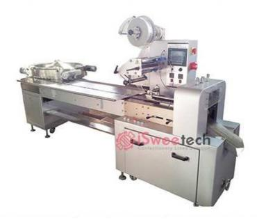
This machine is suitable for simple-grain hot pillow type packing of the candy. It adopts frequency conversion activator to adjust the speed, and equipped with a photocell to track the color mark, low noise, and high speed.
