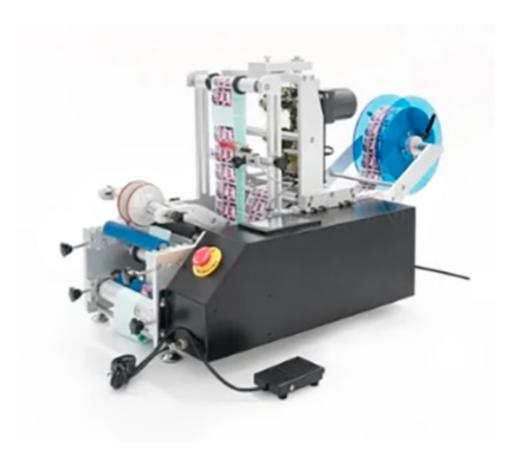
The T-41311 semi-automatic round bottle labeling machine is an efficient cylindrical object labeling machine, which can be applied to cylindrical objects of various specifications, such as xylitol, cosmetic round bottles, etc. Our labeling machine is equipped with full/half-circumferential labeling and circumferential front and back labeling functions, which can meet the labeling needs of different products.
