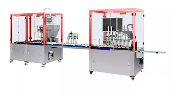
Integrate with air cleaning, filling, inserting, capping and outlet function, suits for fill the water injection, lotion and cream products. This machine adopts the double line program air cleaning, filling, capping and outlet.
