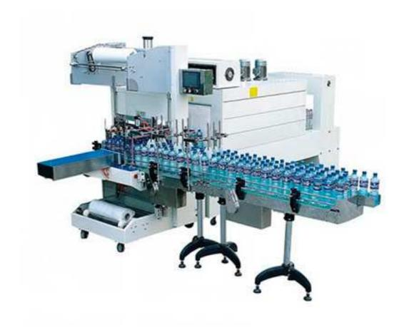
Shrink packing machine for packaging production of beer, beverage, pure water, fruit juice, dairy product, etc. With full automatic functions Bottle entering→ Auto unscrambling bottle→ Pushing bottle→ Heat sealing-Cool cutting →Pressing PE→ Shrink→ Cooling.
