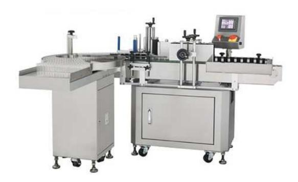
AL505 Vial Labeling Machine is specialized in vial labeling or other small round bottles. When labeling, the ampoule will automatically rotate to allow the labeling device to apply the pressure for labeling. Suitable for medicine, food, beverage, and chemical industries. Can be used for plastic, glass, metal and other round containers/bottles. With its innovative design, its operation is so simple that even a primitive man can use.
