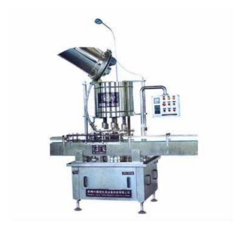
FXG-6/8B rotary automatic capping machines, is in the absorption of foreign advanced technology, based on the ideal of improving the design of the new cap equipment, it has: small size, transmission structure is simple, smooth operation, low noise, using the range, cap rate, handsome in appearance and so on. For pesticides, alcohol, medicine, beverage, chemical industry, glass, polyester bottles, automatic rotary joint sealing work.
