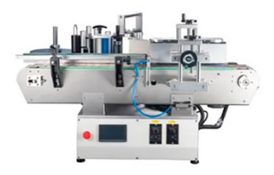
This labeling machine is specially designed and specific, and is dedicated to labeling round bottles provided by customers. After being familiar with this equipment, it can be applied to the round bottle labeling of other products.
