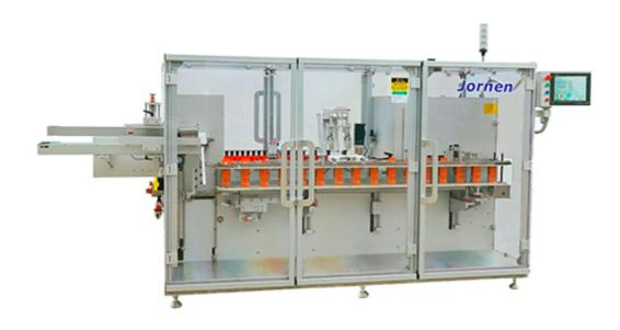
Vertical Cartoning Machine ZV60 is a mechanically driven, intermittent motion vertical cartoner, it is suitable for packaging cosmetic and pharmaceutical products that require vertically loading into a carton at speeds of up to 60 cartons per minute.
