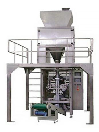
The full-automated VFFS small bag filling machine is designed to realize the fully automatic operation of metering, material feeding, bag making, sealing-off as well as coding.
