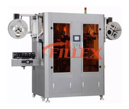
This Shrink Sleeve Labeling Machine adopts international advanced technology, cover the circle label on the PET bottle, and then hot shrinking to fix on the position which bottle body designated. The machinery part adopts combination designing of modularization, and makes the machine reasonable. The height adjustment adopts motor fluctuating, it is convenient to replace the material. The special cutter head designing, make the film-rolling cut mor exactly and reliably.
