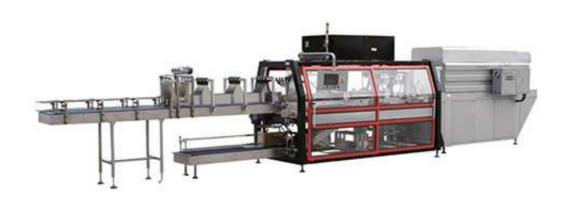
This machine mainly use for bottle and cans packing processing, it is 2 in 1 automatic packing machine, can tray carton forming, packing, film wrapping then shrinking.
