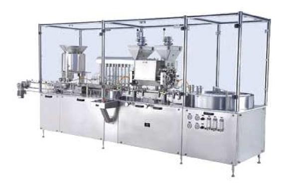
SBML-300D, is a monoblock type high speed machine which has injectable dry powder filling, vial liquid fillig & rubber stoppering machine in one frame structure.
