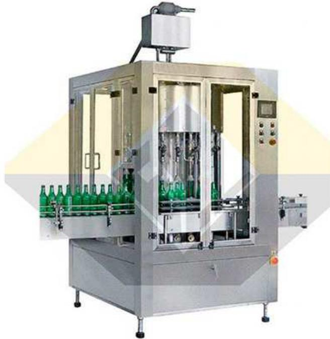
VFL-20X Automatic (Gravity) Liquid Filling Machine is the most advanced rotating filling machine for liquid in our country. It is suited for gas (carbonated) products. Like beverage/bottle water, juice, alcohol, sauces, edible oils, especially for the chemical, emulsion, pesticide, etc. The filling volumes range is 30ml - 1000ml, the max filling speed can reach 7000 bottles/hour.
