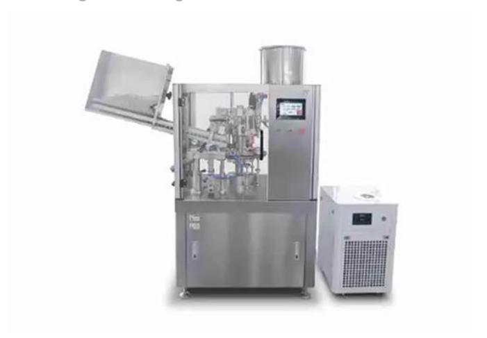
This equipment is widely used in daily chemical, pharmaceutical, cosmetic and food industries, and is suitable for various materials such as ointment, cream, gel or viscous fluid. It can automatically complete a series of actions such as tube loading, label identification and positioning, tube internal cleaning (optional), filling, tail heat melt sealing, coding, shearing, and finished product output.
