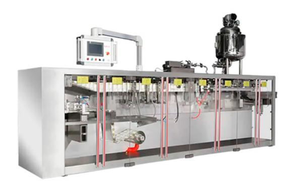
BHD-130S is specially designed for the needs of stand-up pouches. The filling capacity is 1-350g. It can be used to package functional drinks, enzyme puree and other liquids. Seventeen work stations ensure the accuracy of filling amount and packaging speed, and are flexible. Functional applications, such as: hanging holes, special shapes, zippers, suction nozzles, etc., can fully meet customers' customized needs.
