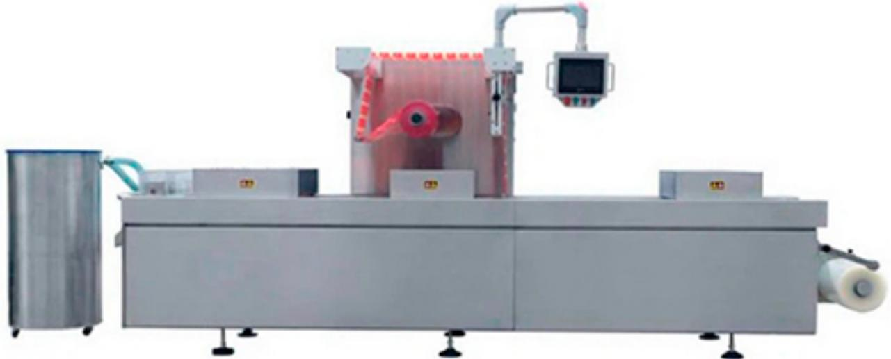
HVR-A Series Automatic Thermoforming Vacuum Packaging Machine can continuously finish the procedure of film forming, automatic or manual products feeding, vacuuming, sealing, cutting, etc.; it will skin pack the product.
