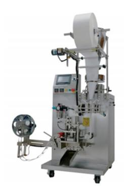
YS-66 machine is suitable for particles material, such as: tea, coffee, food, medicine and chemical products. Lean machine concept enables cost-effective production. All the works of bag making, measuring, filling, sealing, cutting and counting can be done automatically. The touch screen operation, PLC control, drive stepper motor to control the bag length, stable performance, easy to adjust and accurate detection.
