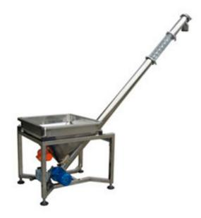
The Machine can convey sorts of material. Combined with the package-machine of our company, it can do material situation tracing. It also can be used separately. Complete machine made in stainless steel, except for the electrical machine, gearing, and the framework.
