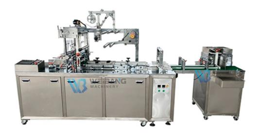
The machine is widely applicable to the automatic film packaging (with gold tear tape) of various single boxed articles.
