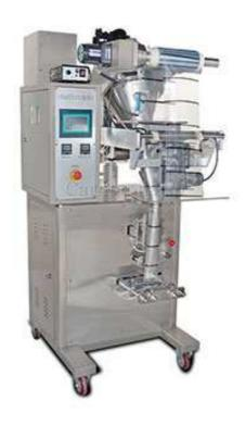
Automatic Powder/Granule packing machine is mainly used packing different kinds of coarse powder, granule material side sealing flat bag or pillow bag filling and packing. Specific materials that can be packed: all kinds of soup powder, seasonng, Chinese patent medicine, coffee, soybean, solt, melon seeds, tea, etc..
