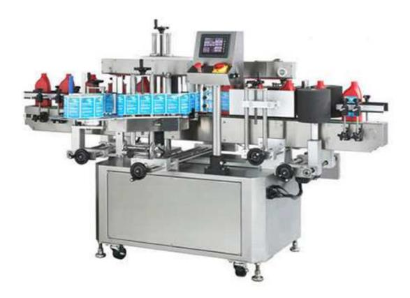
With the comprehensive industry knowledge of allied domain, we are engaged in presenting a superior quality range of Automatic Labeling Machine. The offered machine is suitable for applying single side labels on flat / round shape containers with output Up to 120 labels per minute depending on products size and label size. Automatic product alignment system synchronized with top holding mechanism. Apart from this, clients can get the machine from us at industry leading rates.
