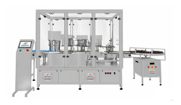
Monoblock Filling Machine is the most demandable system for pharmaceutical manufacturing businesses. Its innovative technology combines the three essential functions into an integrated unit, paving the way for seamless packaging. Harikrushna Machines Pvt. Ltd. offer a cutting-edge machine to streamline your liquid filling, inner plugging, and capping processes with unmatched efficiency and fulfil the speed and precision requirements at a budget price.
