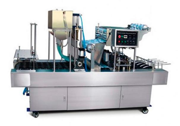
BG32P (2 cups)/BG60P (4 cups) automatic cup filling and sealing machine is widely used in filling and sealing various kinds of plastic cups for sticky liquid and paste material.
