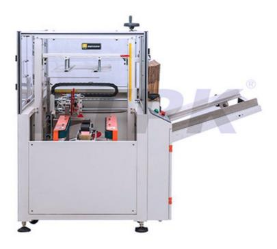
Vertical storage is adopted for storaging carton blanks, for which carton blanks can be added at any time without stopping the machine;
