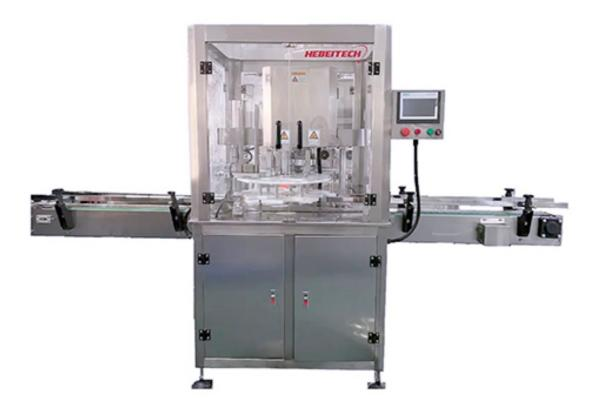
This automatic can seaming machine or called can seamer is used to seam all kinds of round cans like tin cans, aluminum cans, plastic cans and paper cans. With reliable quality and easy operation, it is ideal equipment necessary for such industries as food, beverage, pharmacy and chemical engineering. The machine can be used alone or together with other filling production lines.
