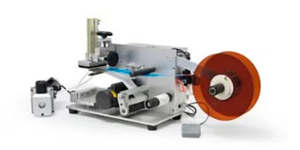
The machine adopts high precision intelligent electric eye and extremely reliable programmable logic controller (PLC) for label peeling, label outputting and labeling. Adhesive labels will be adsorbed to the labeling head by air pressure, and then will be labelled on the item.
